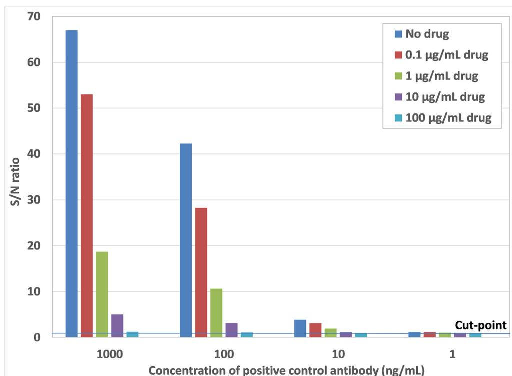
Figure 2: Graph from case study showing the assay sensitivity in the absence and presence of several concentrations of drug. The assay sensitivity is between 1 and 10 ng/mL anti-drug antibodies, which is well below the regulatory required sensitivity of 100 ng/mL. The drug tolerance is between 10 and 100 µg/mL of drug at an anti-drug antibody concentration of 100 ng/mL.
