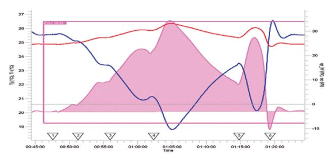
Metallic zinc was added in six portions (each addition is depicted by a triangle on the X-axis) at 25°C. The energy release was instantaneous (pink surface) and by applying cooling (blue line) the reaction temperature (red line) was maintained at 25-26°C. This approach enabled full control over this highly exothermic reaction and was successfully applied at 20-litre scale in our plant.
