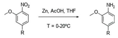
To ensure safe processing, our chemists proposed alternative conditions for this step. The working hypothesis here was that portion-wise addition of zinc at elevated temperature would enable better control over the temperature rise associated with the heat released during the reaction. An experiment in the reaction calorimeter was set up to test this hypothesis (see figure below).
