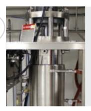
Capacitymg to kgFlow rates1-4000 mL/minColumn diameter5-300 mmTemperature5-60°CPressure≤ 100 bar
